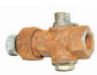
CAST IRON PLUG After 12 Hours
