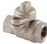
T.E.A. COATED VALVE After 250 Hours
