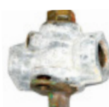
GALVANIZED PLUG After 30 Hours
