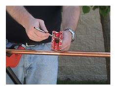
**Step 3**Apply a liberal amount of the provided gasket sealant (Loctite 518) and brush evenly across the entire body half surface.
